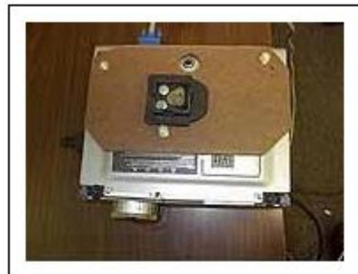
The figure to the right shows a projector with its mounting plate attached.
