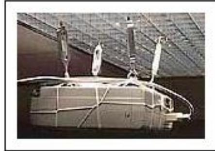
slightly: Its the projectors are not turned sideways. One is on top of a bookshelf and the other hangs upside-down from hooks in the ceiling, as shown to right, demonstrations of the ways one can (and often must) improvise when accommodating a CaveUT setup to its environment.
