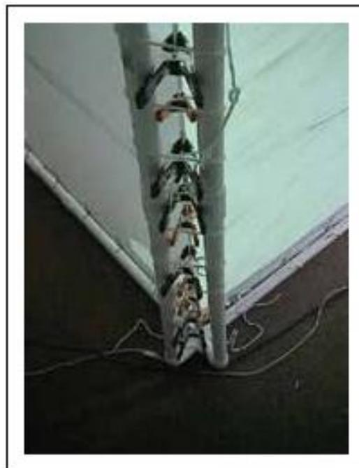
One by one, put the metal clamps into place, so the seam looks like the one shown in the illustration to the right. While doing this, make sure that the edge of the two screens is pulled taught. At this point in the process, there will be creases and wrinkles in the screen material, and it's important that no creases or wrinkles remain between the seam binders.
