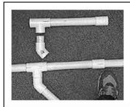
picture to the right illustrates how those two diagonal cross pieces attach to the frame. The cross-pieces are only needed to increase the strength and stability of the frame. The picture to the right also shows how the very short pieces of PVC pipe fit the joiners together into larger configurations.
