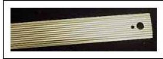
A "carpet seam binder" is a strip of metal (as shown to right) which is sometimes used in the United States to cover a seam between two carpets, especially if they are of different types or there is a gap between them. With the V-Cave, carpet seam binders were used to clamp the edges of the two screens together at the corner where they join, as shown to the left.
