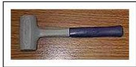
Avoid the black hard-rubber mallets. They smell bad, leave black marks on the pipes, and tend to become damaged by use.
