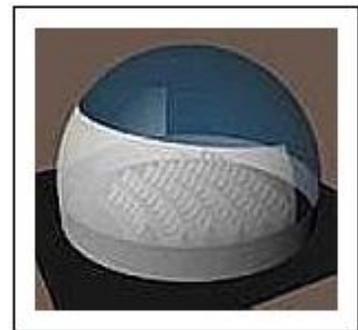
On the right is a Schematic of the Earth Theater. The screen is a section of a sphere, 210 degrees horizontal by 30 deg vertical. In the figure, the screen is depicted in a transparent white in front of the seats.
