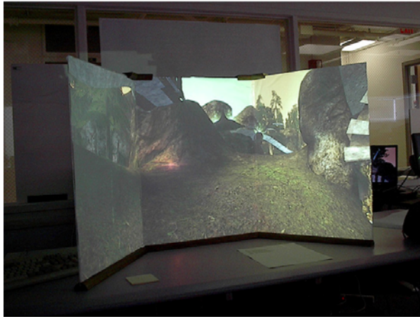
Figure 2: (left) The MiniCave, desktop-sized immersive display intended for a seated observer. (right) An overhead-view schematic of the MiniCave.
